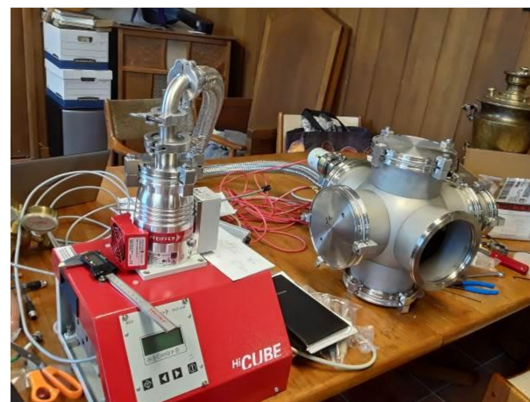
Fig. 3. Pumping system for self-focused ion beam, production
