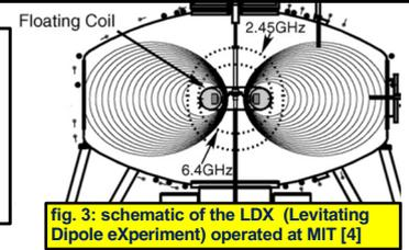
fig. 3: schematic of the LDX (Levitating Dipole eXperiment) operated at MIT [4]
