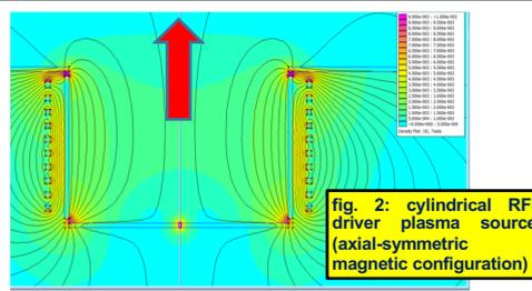
fig. 2: cylindrical RF-driver plasma source (axial-symmetric magnetic configuration)
