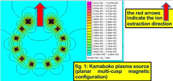
fig. 1: Kamaboko plasma source (planar multi-cusp magnetic configuration)
