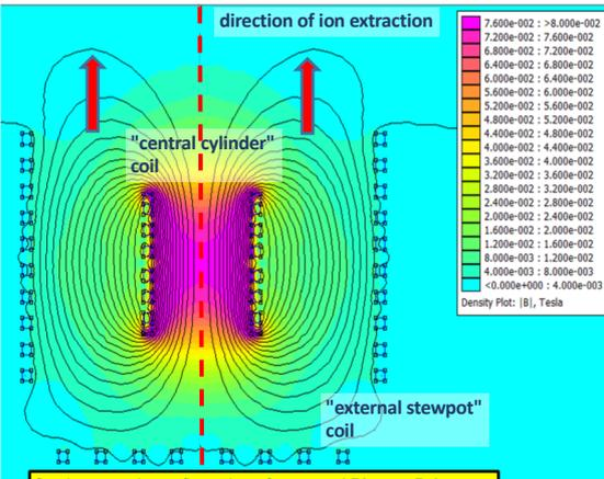
fig. 4: magnetic configuration of proposed Plasma Driver (axial-symmetric geometry)
