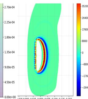
fig. 9: plasma diamagnetic current density obtained by solving the Grad-Shafranov equation
