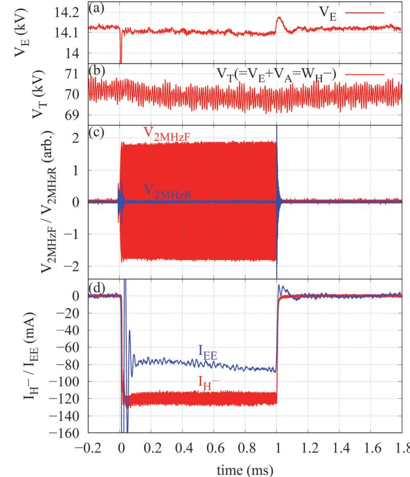
Waveforms of  $V_E$ (a),  $V_T$ (b),  $V_{2MHzF}$  and  $V_{2MHzR}$ (c) and  $I_{H^-}$  and  $I_{EE}$  (d) of one beam pulse. \*Flat  $I_{H^-}$  by tilting up  $P_{2MHz}$  by 9% to comp.  $V_E$ & $V_T$  droops.
