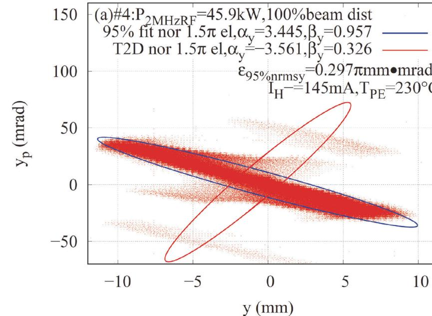
100 % beam  $H^-$  ion distribution (red dots), fitted normalized  $1.5\pi\text{mm}\cdot\text{mrad}$  ellipses fitting 95% beam (blue line) and ellipse backward traced to GE downstream surface with TRACE2D (T2D) (red line) in horizontal (a) or vertical (c) phase-plane.
