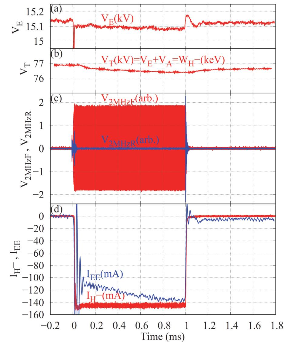
Waveforms of  $V_E$ (a),  $V_T$ (b),  $V_{2\text{MHzF}}$  and  $V_{2\text{MHzR}}$ (c) and  $I_{H^-}$  and  $I_{EE}$  (d) of one beam pulse. \*Flat  $I_{H^-}$  of 145 mA was produced with 0.9% tilting up P2MHz.
