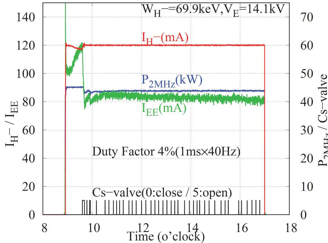
Trend graph of  $I_{H^-}$ ,  $I_{EE}$ ,  $P_{2MHz}$  and  $Cs\text{-valve}$  close/open during **8 hours operation**, in which  $I_{H^-}$ , was feedbacked to  $120 \pm 1 \text{ mA}$  by  $P_{2MHz}$ , for  $W_{H^-}$  and  $V_E$  of  $69.9 \text{ keV}$  and  $14.1 \text{kV}$ , respectively. In station. state,  $Cs$  inject. rate =  $42.3 \mu\text{g}/\text{hour}$ .
