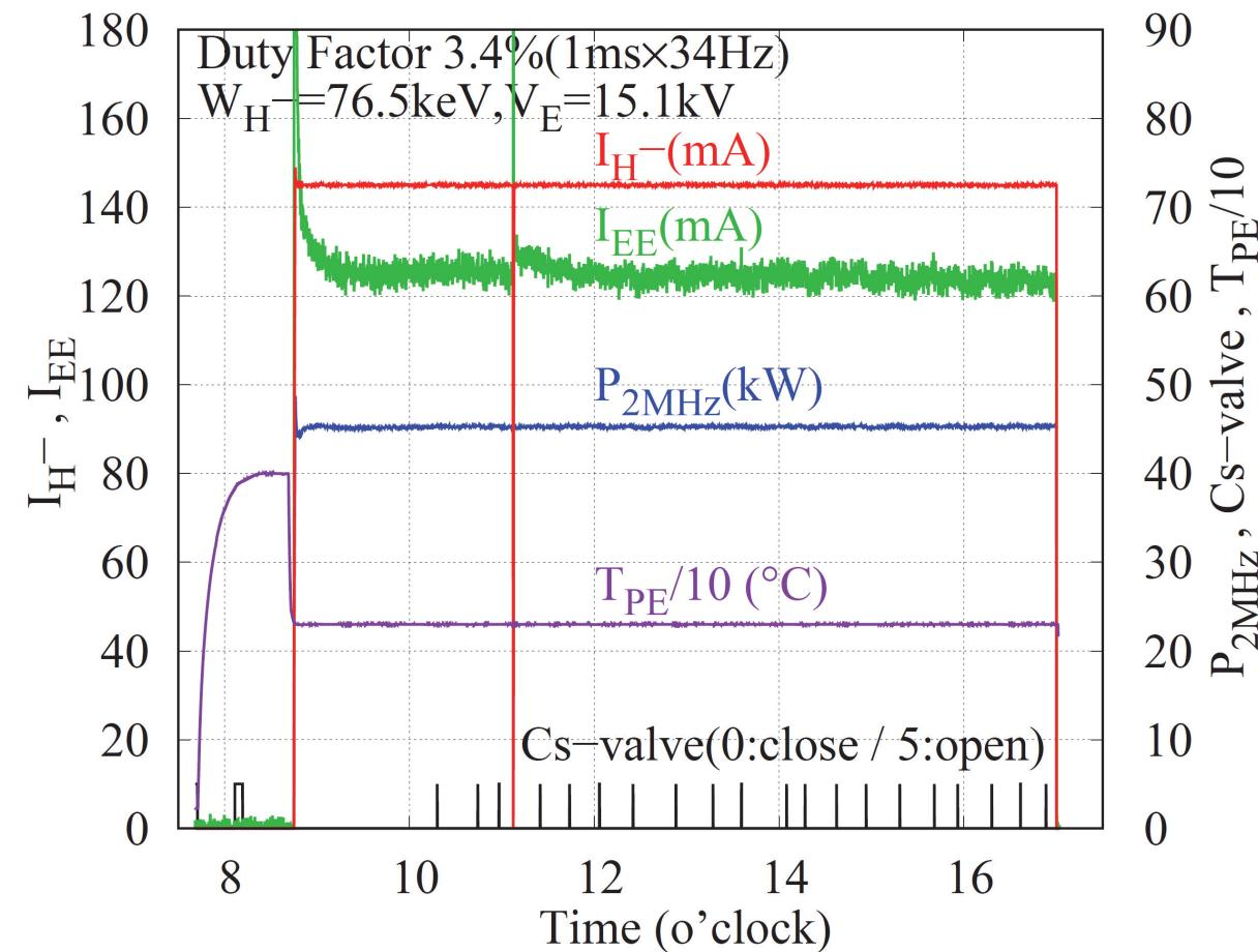
Trend graph of  $I_{H^-}$ ,  $I_{EE}$ ,  $P_{2\text{MHz}}$ ,  $T_{PE}$  and Cs-valve close/open during 8 hours operation, in which  $I_{H^-}$ , was feedbacked to  $145 \pm 1 \text{ mA}$  by  $P_{2\text{MHz}}$ , for ( $W_{H^-}$ ,  $V_E$ ,  $T_{PE}$ ) of (76.5 keV, 15.1 kV, 230  $^\circ\text{C}$ ). In stational state, Cs inject. rate = 14  $\mu\text{g}/\text{hour}$  < 42  $\mu\text{g}/\text{hour}$  for 69.9 keV 120 mA @  $T_{PE}=245\text{ }^\circ\text{C}$ .
