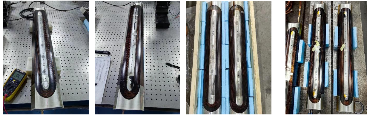
NbTi sextupole coils
