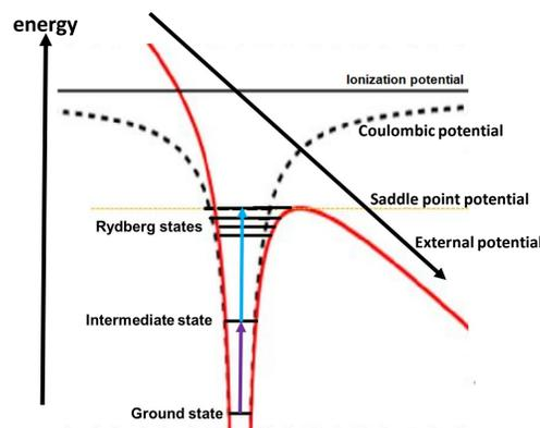
The saddle point model of electric field ionization. An external potential deforms the atom's potential well, creating a saddle point that allows the electron to escape.
