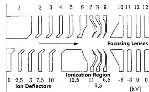
Stacked electrodes design with ion filter and spherical potential for beam focusing and energy labelling [2]. This design is open to atom/ion beams.
