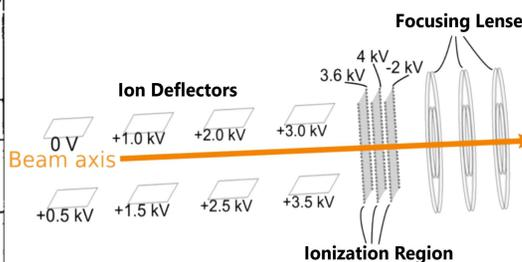
Mesh grid design producing a uniform electric field with minimal focusing [3]. A high transparency grid is required, which will be subject to interaction with the atom/ion beam.
