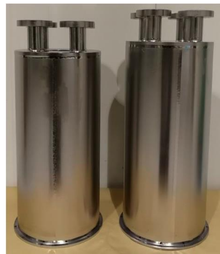
Photo of Coaxial Cavities: HWR (left) and QWR (right)
