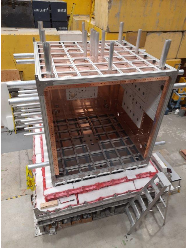
Copper shield and structure (Feb. 2023 status)
