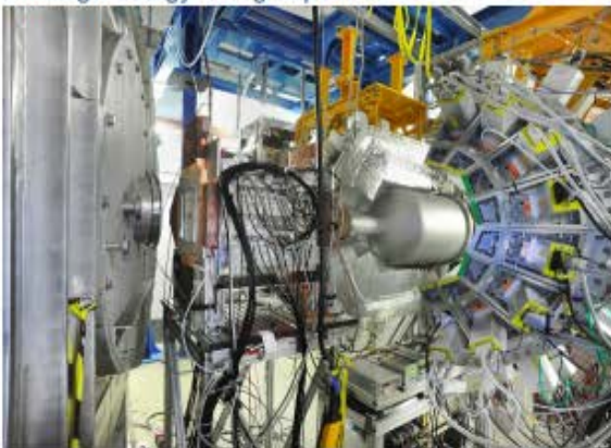
CALorimeter for In-Flight detection of \gamma -rays and high energy charged particles
