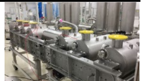
Cold mass assembly in clean room
