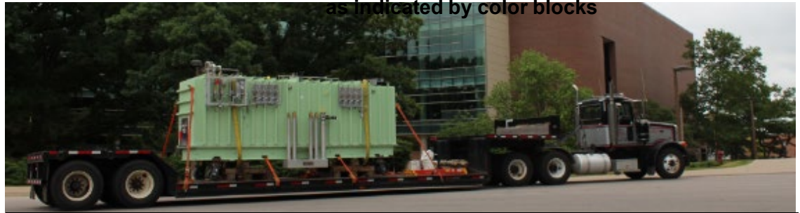
Forty-sixth and final baseline cryomodule (eighteenth \beta=0.53 cryomodule) being transported to the tunnel
