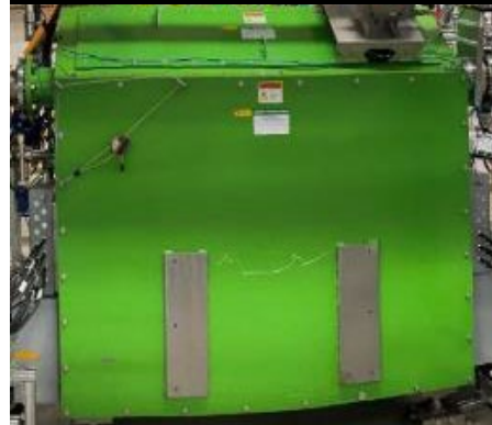
Liquid lithium charge stripper installed in FRIB tunnel
