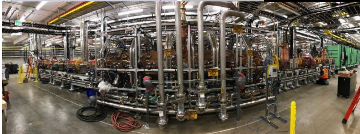
FRIB Lower LEBT, RFQ, MEBT, and the three \beta=0.041 cryomodules installed
