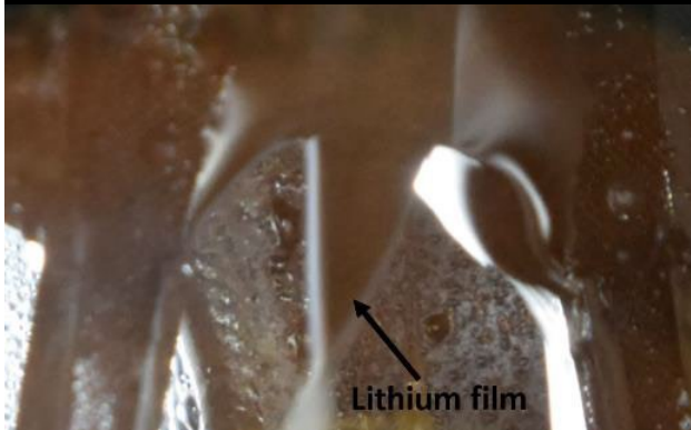
Melted liquid lithium film as seen from a view port in the charge stripper
