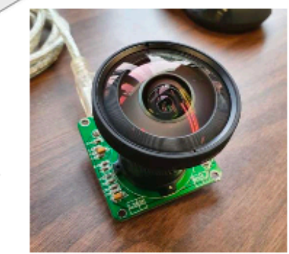
Fish-eye lens camera for monitoring bioluminescence and sedimentation
