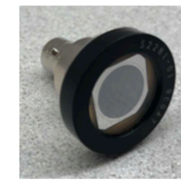
Photodiode and silicon photomultiplier used for flash self-monitoring
