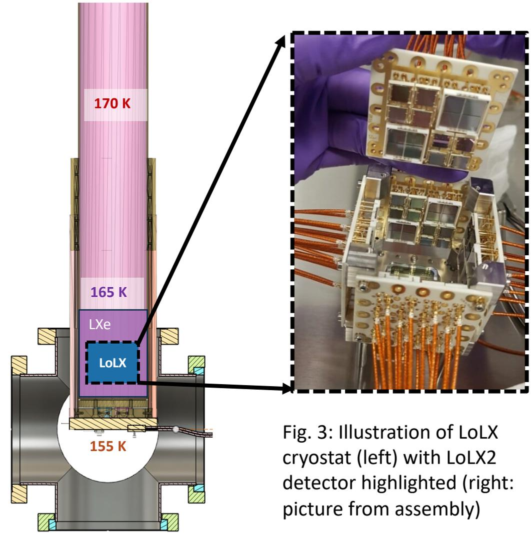
Fig. 3: Illustration of LoLX cryostat (left) with LoLX2 detector highlighted (right: picture from assembly)
