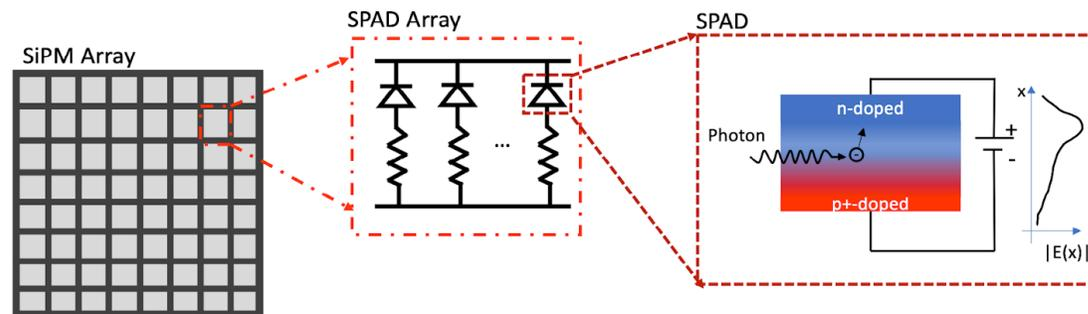
FIGURE 2.10: Illustration of SPADs modelled as a P-N junction within a SiPM array with each channel corresponding to an individual SiPM. Each SiPM is then composed of many such SPADs. Photons ionize atoms in the SPADs depletion region, creating an avalanche of charge that is then readout.
