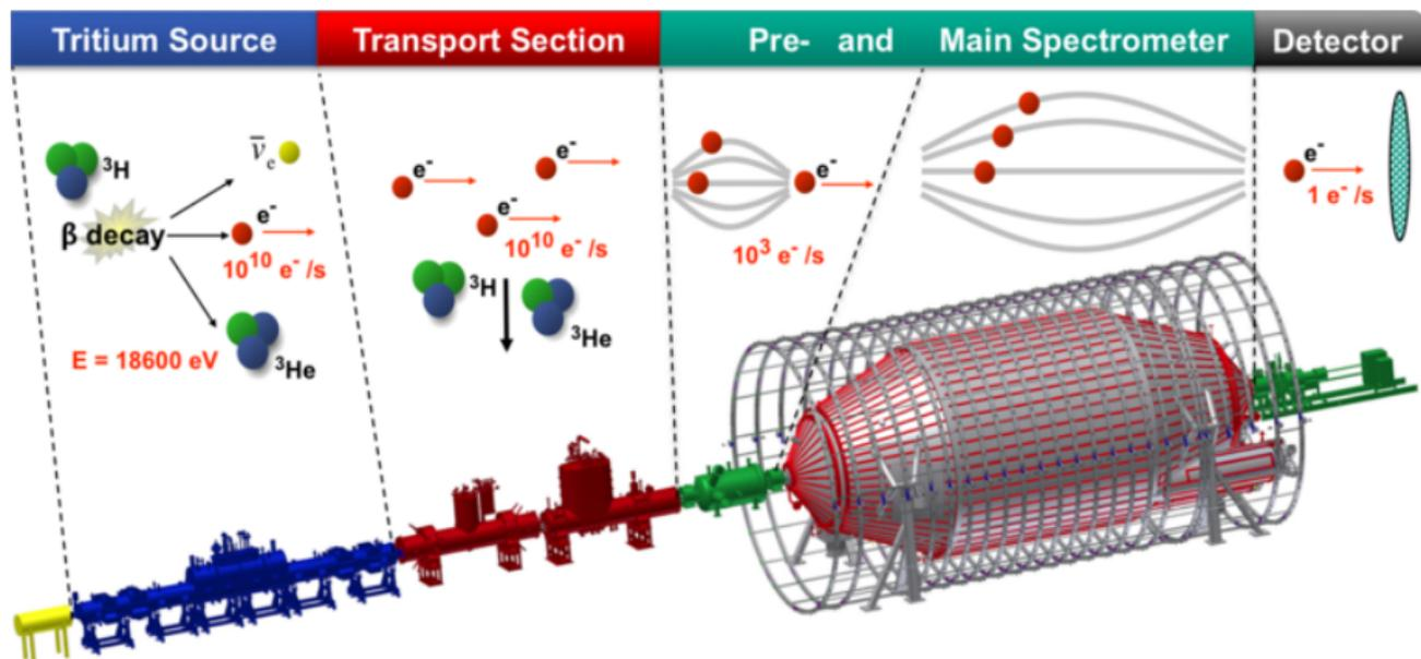
Tritium decays, releasing an electron and an anti-electron-neutrino. While the neutrino escapes undetected, the electron starts its journey to the detector.
