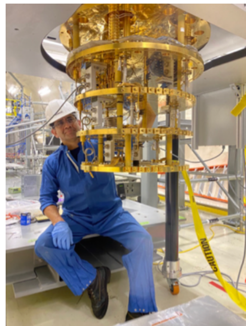
Standalone test of the dilution fridge demonstrated base temperature
