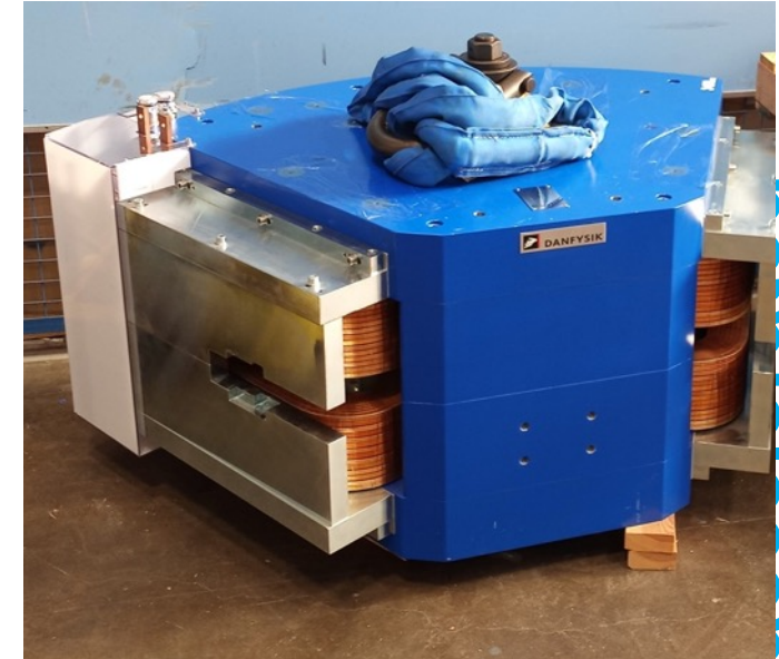
RIB beamline pre-separator
