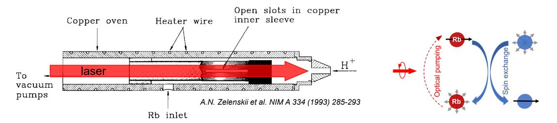
Similar configuration as the optically-pumped polarized H<sup>-</sup> ion source designed at TRIUMF previously. H<sup>+</sup> passes through optically pumped Rb vapor in a neutralizer cell and picks up polarized electrons by charge exchange to form electron-polarized neutral H atoms.
