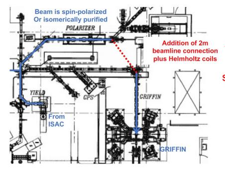
beamline extension for polarized beams to GRIFFIN spectrometer (2027)
