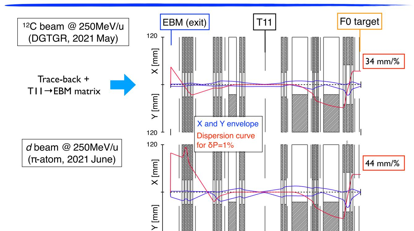
♦ Different dispersion curves at SRC exit were observed for different beams !
