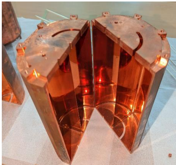
“Pizza” Cavity is divided into subregions and read out coherently. S. Youn, CAPP (2023)
