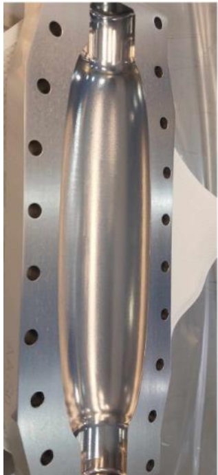
SQMS at Fermilab reports a Q of 10^6 with NbSn -R. Cervantes, Patras 2023
