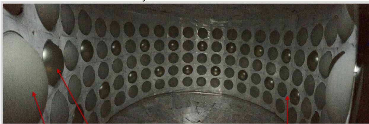
TPB coated PMTs Uncoated PMTs
