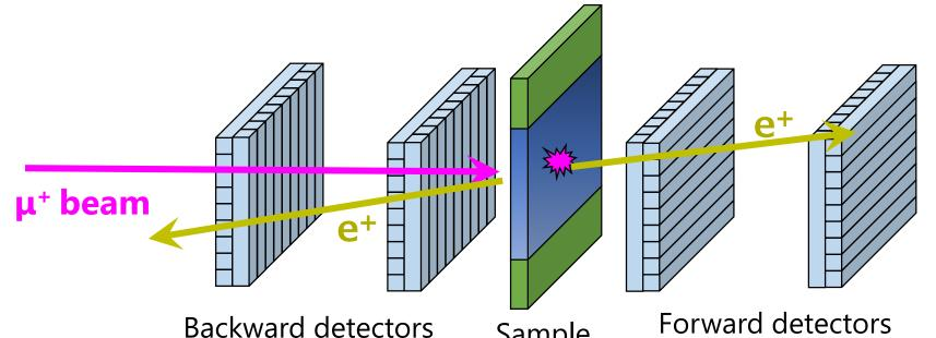
Concept of detector layout for µSR measurement
