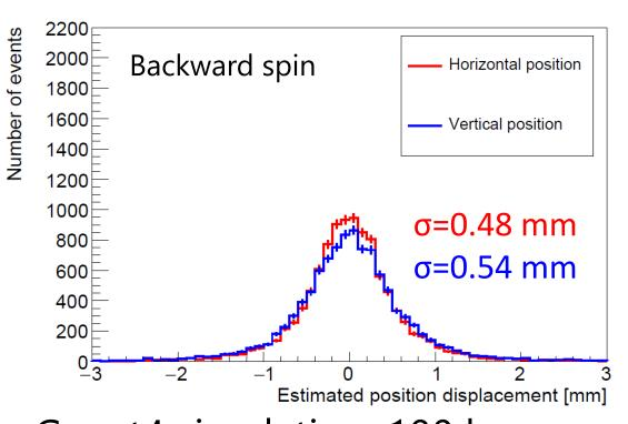
Estimated position displacement from Geant4 simulation. 100 k muon decay events were simulated for each condition.
