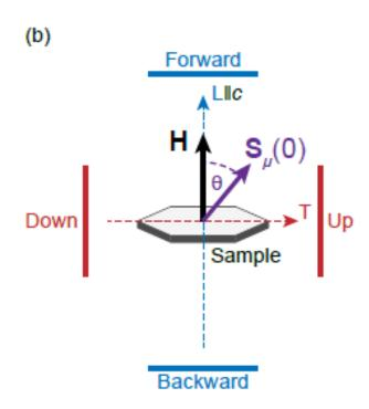
Spin rotator measurements using GPS at PSI
