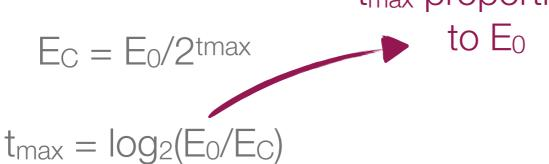
$t = X/X_0$   $X_0 = \text{radiation length}$  $E_0 = \text{initial energy}$
