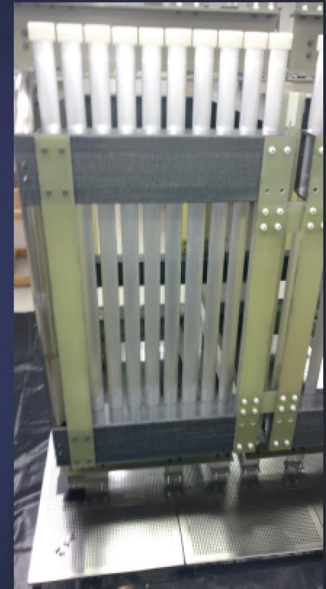
Field cage made out of Al extruded profiles
