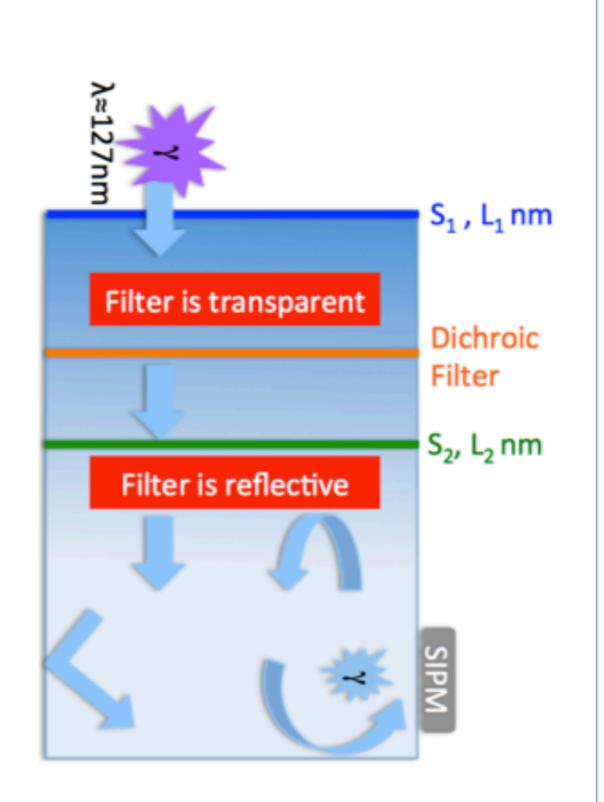
ARAPUCA allows to have a reasonably high light detection efficiency (few percent) on large areas (hundreds of cm<sup>2</sup>) with a limited coverage of active components (SiPM). These properties make it particularly suited to be used in large liquid argon Time Projection Chambers, like the **DUNE experiment**.
