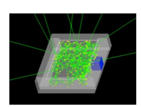
A full Monte Carlo simulation of the **ARAPUCA** was developed. It is based on the Geant4 package, and it takes into account all the main optical properties of the constituting materials.
