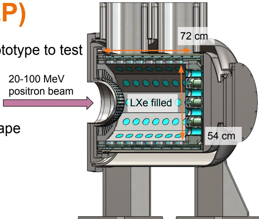
Current large prototype design using ~650 kg of LXe. Nominal design has 133 photomultiplier tubes (PMTs) and 400 silicon photomultipliers (SiPM) quads.
