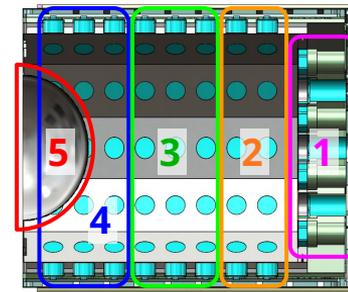
The weighting of photon hits is needed because of the different PMT/SiPM coverage on each surface.
