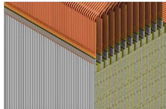
Design baseline: 48 stacked planes of  $120$   $\mu\text{m}$  thick AC-LGAD strips
