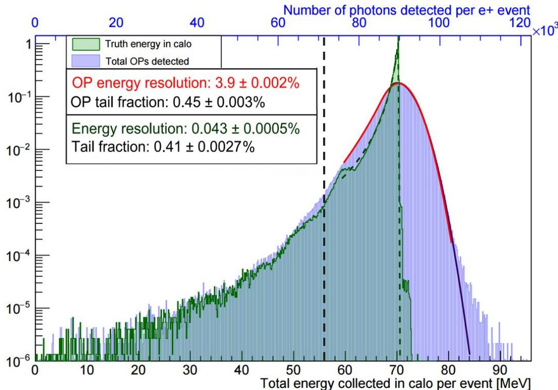
LP simulation results for  $5 \times 10^6$  positron events
