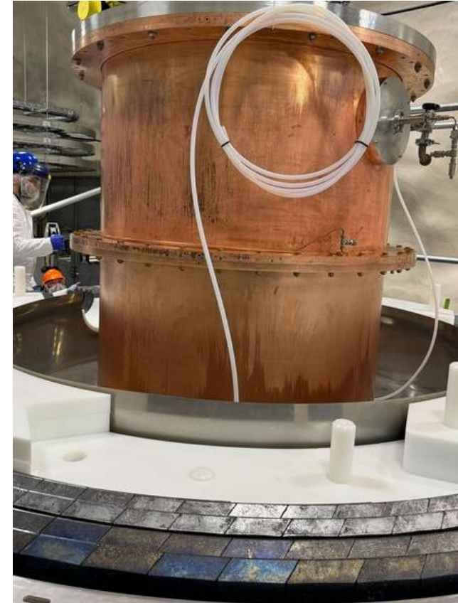
Outer cryostat can, placed on the bottom of the shielding
