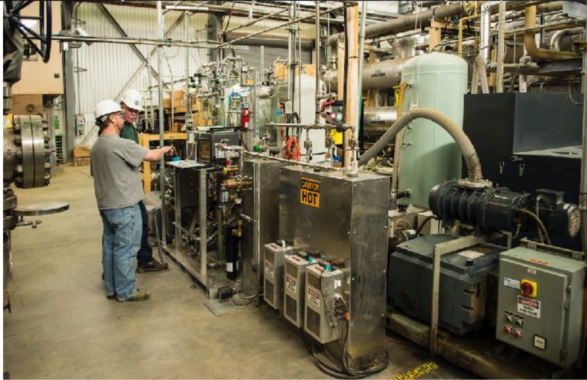
Picture of the extraction plant used to procure DS50 UAr target (<0.5kg/d)
