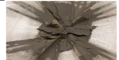
Fig. 4: Filtered deposits of various copper oxides flushed out of QWB8, the last quadrupole magnet in the injection beam line. The pore size of the filter is 12 μm. The dry weight of the residuum amounts to 0.72 g.
