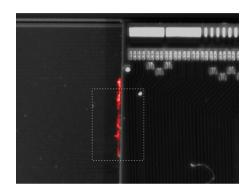
Identifying the location of a sensor breakdown using hot spot imaging
