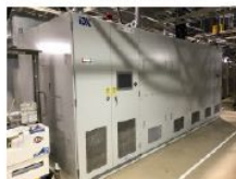
New Horn PS/trans/ strip-lines for 320kA & 1Hz
