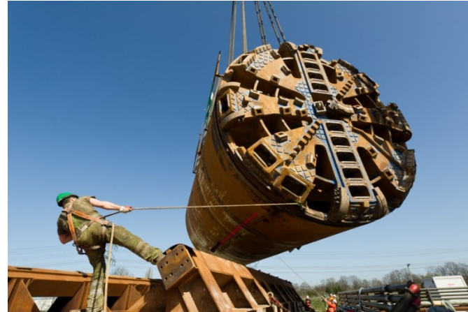
Removing the cutter head \varnothing 5.3m
