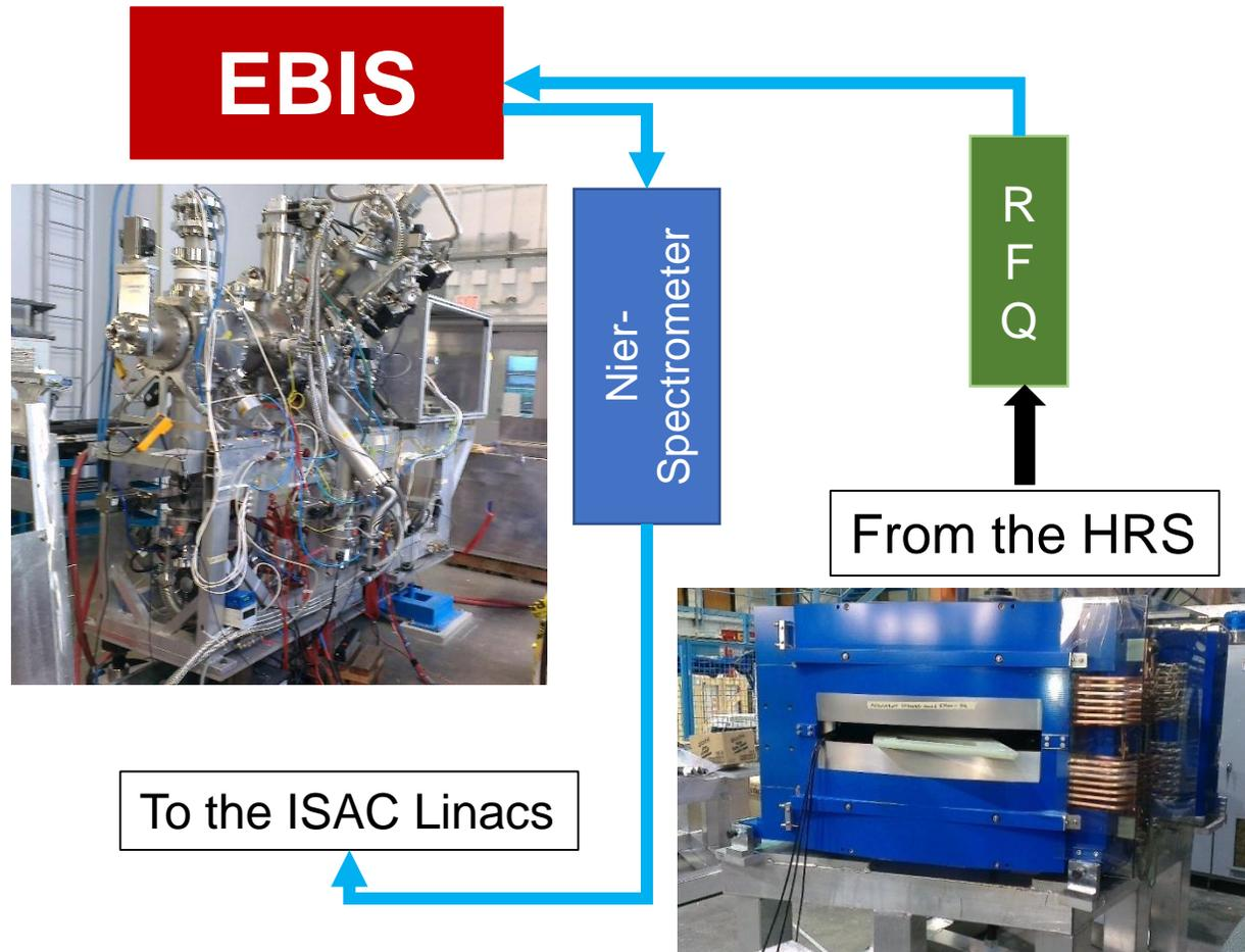
CANREB (funded CFI project, SMU) is the unique beam preparation system for high quality ARIEL beams:
