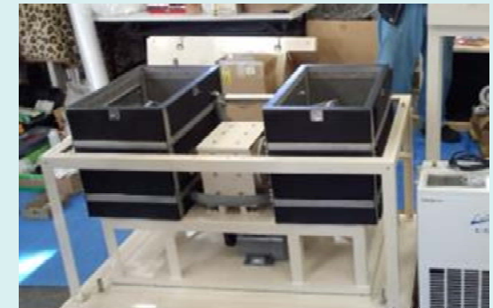
Mechanical Alloying in vac.
