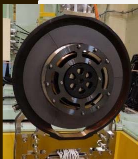
Muon Target @MLF, J-PARC 3 GeV, 1 MW Graphite target
