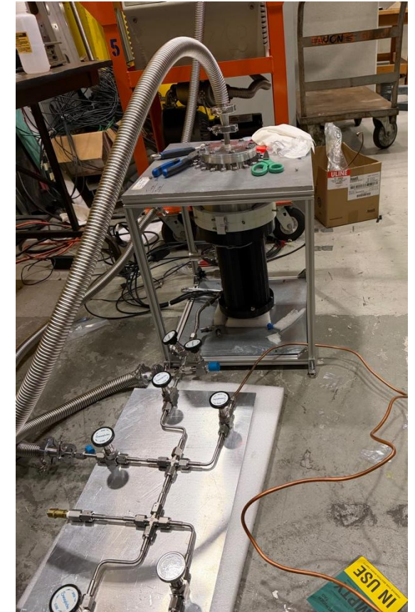
Filling of detector with \text{CF}_4 and ^3\text{He} gases
