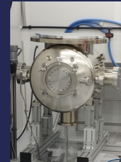
Gun chamber HPR cleaning in clean room
