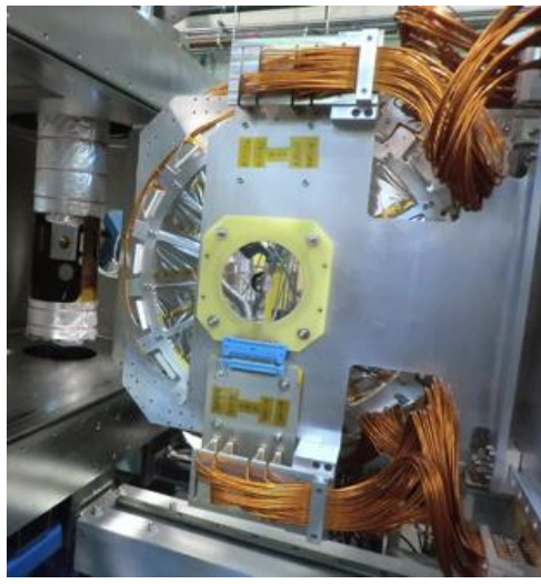
IRIS Solid hydrogen target for direct reactions
