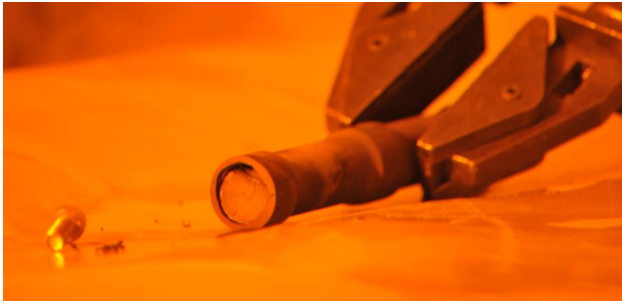
Post-irradiation inspection of a UCx target in the hot cell
