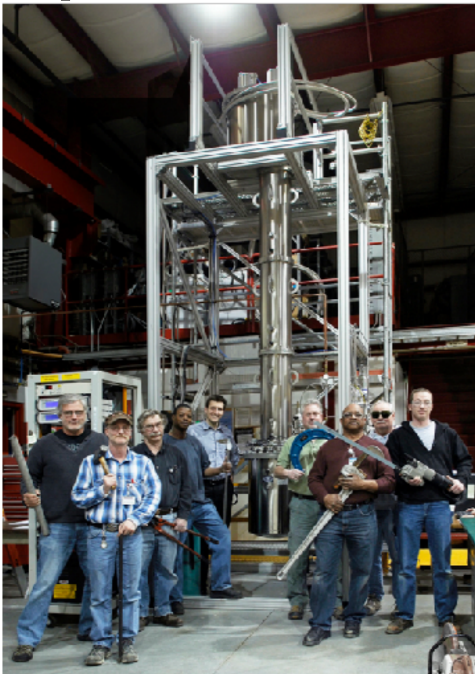
Cryogenic distillation column for purification of ^{39}\text{Ar}
