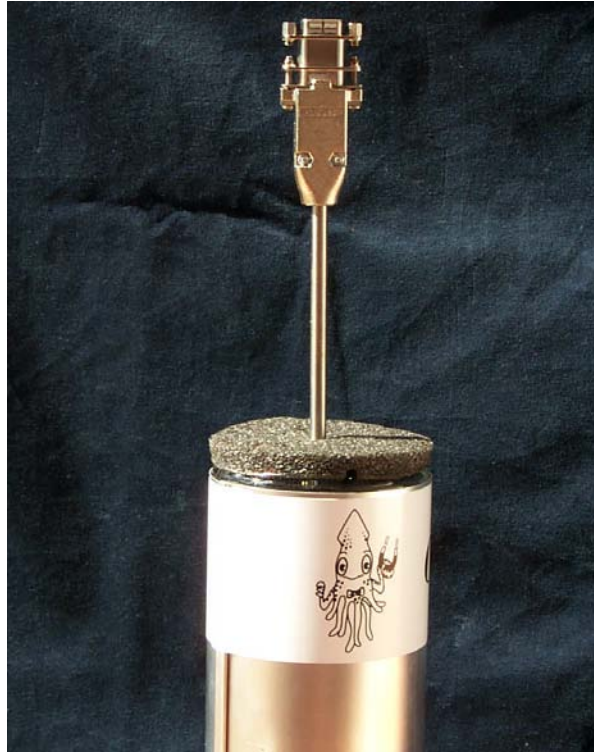
Figure 3-3 Mr. SQUID ® probe inserted into the liquid nitrogen dewar.
