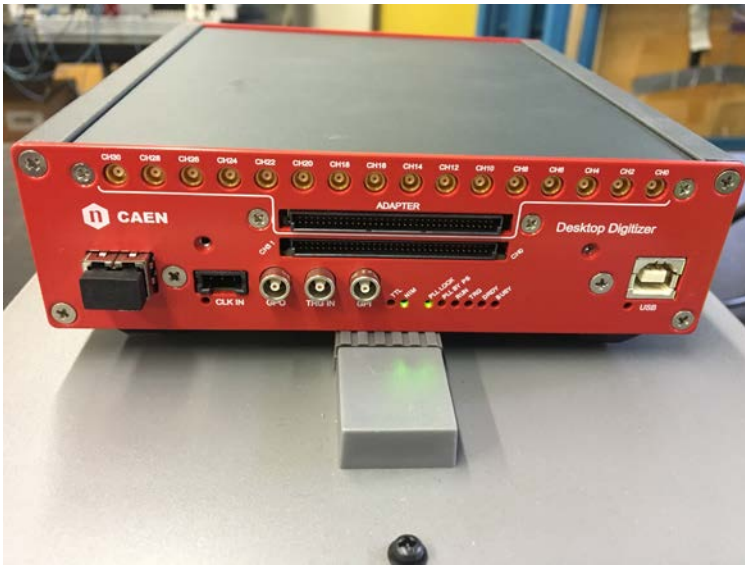
Figure A2.3 CAEN 5740 32 channel 12 bit 62.5 MHz digitizer module.
