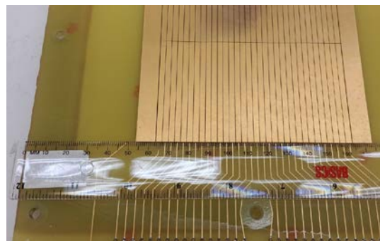
Figure 11 View of anode strips showing the pitch dimension.
