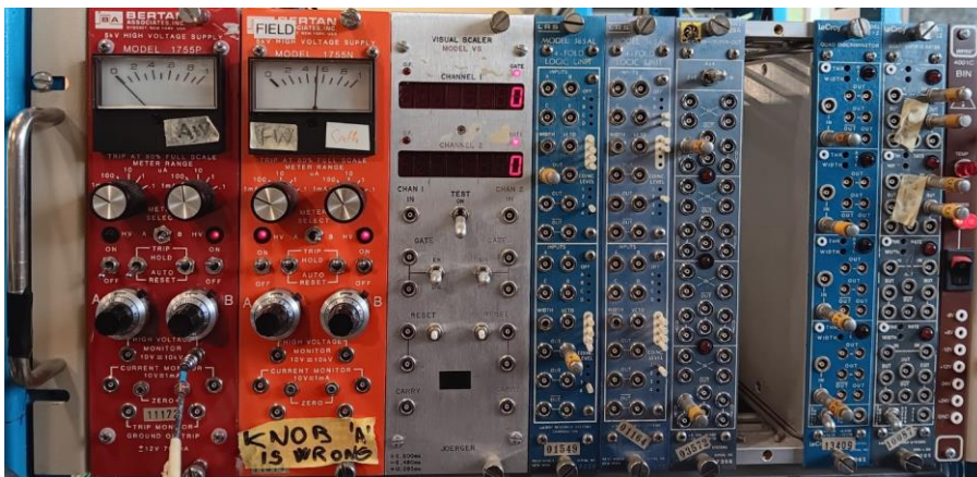
Figure 9 Snapshot of the NIM electronics crate that be used to process the TPC and SiPM signals, next to the high voltage power supplies used for the cathode, anode wires, and field wires.
