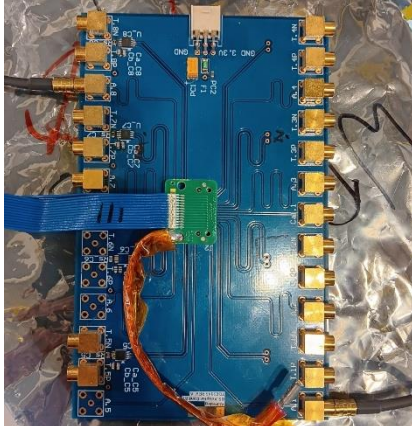
Figure 8 Adapter card between SiPM preamplifier and oscilloscope.
