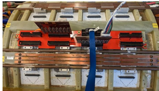
Figure 7 Readout board for the cathode pads with preamplifier, so that the readout is similar to the wires.
