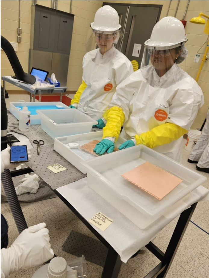
Surface etching removes surface contamination.
