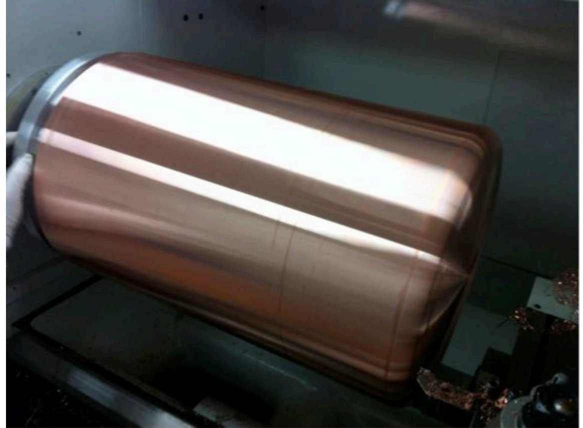
Electroformed copper after turning on lathe.
