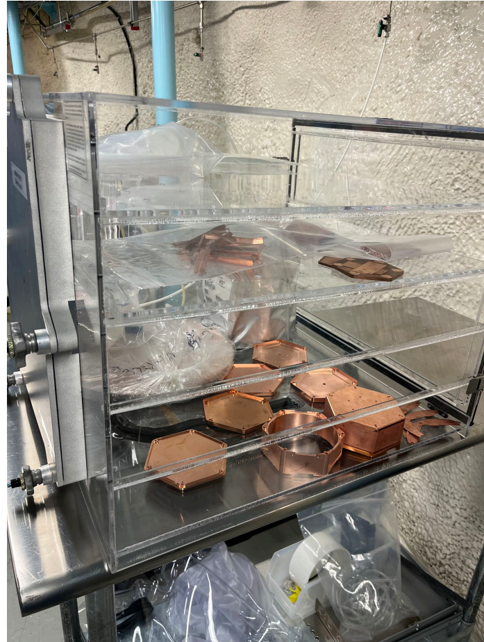
N_2 purge storage to prevent alpha plate out.
