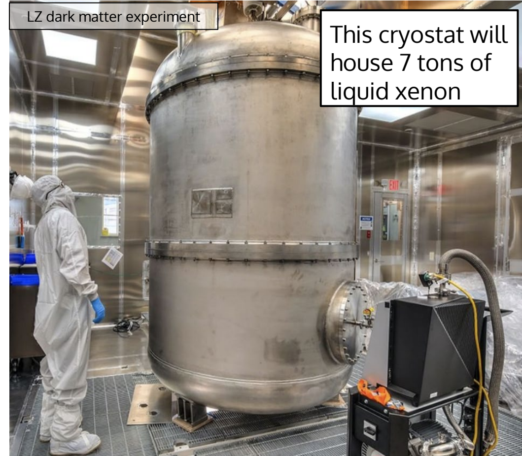
Tight cleanliness requirements for fabrication and assembly → gets more challenging for large experiments.
