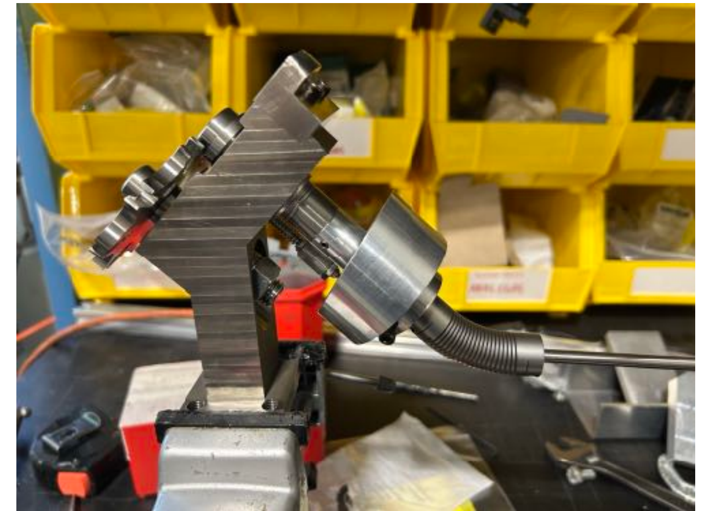
New Geneva Mechanism for Disk Rotation
