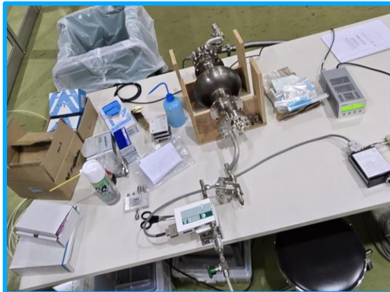
Initial assembly of the plasma processing stand with a single-cell cavity.
