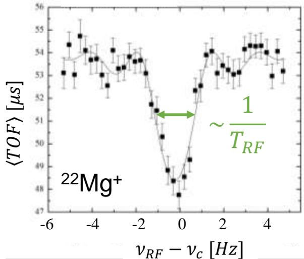
$$\frac{\delta m}{m} \propto \frac{m}{q e B T_{RF} \sqrt{N}}$$
