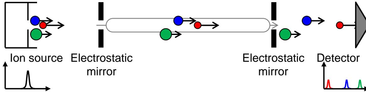
Separation increases with flight path  $\rightarrow$  longer path length
