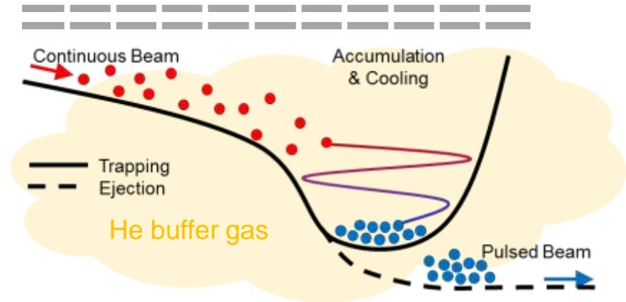
Broadband, fast mass measurements are performed in the MR-TOF-MS.
