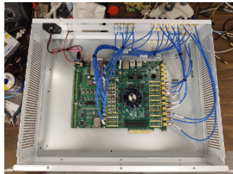
Digital signal processing module hardware
